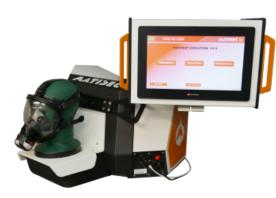
The MATITEST EVOLUTION is a test bench used to verify the proper functionning of open-circuit insulated respiratory systems.
